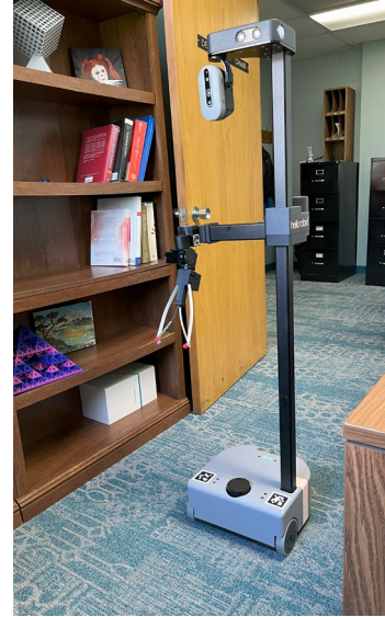
Figure 3. Stretch-2 mobile robot used to evaluate HybridNAV
